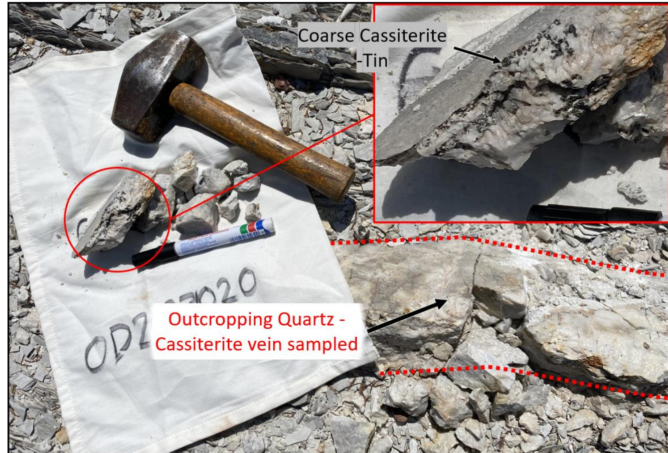
Undrilled quartz vein averaging 2.10% tin with visible coarse cassiterite-tin mineralisation at the Tallebung Project.
