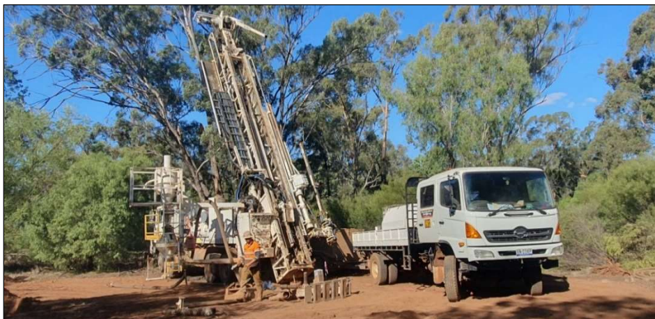
Figure 1: Tallebung Tin Project – RC drilling rig onsite at the Tallebung Tin Project.
