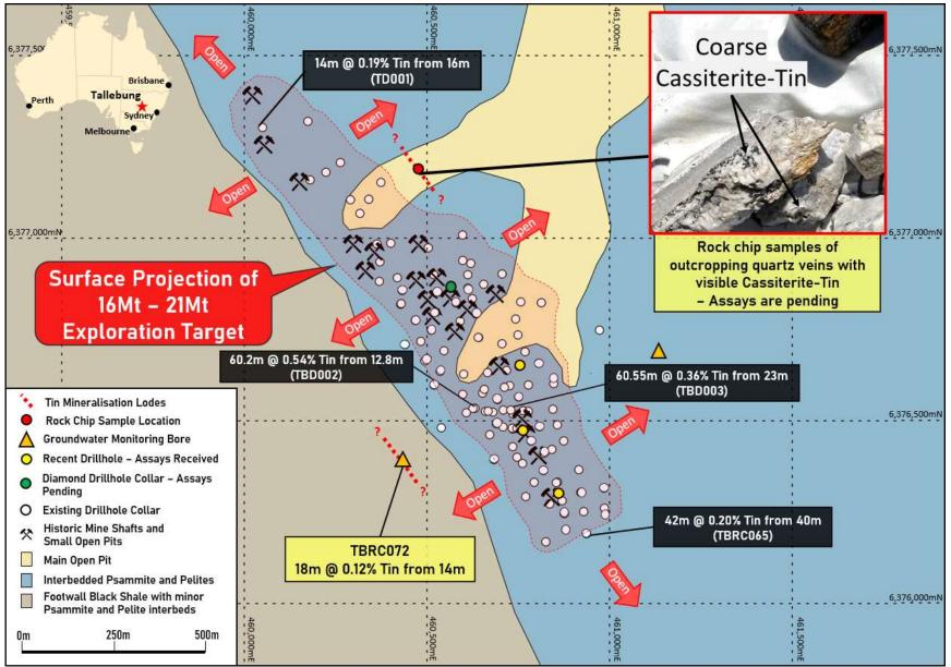
Figure 1: Tallebung Tin Project – Plan showing extent of the current Exploration Target along with the identified extensions to the mineralisation with the tin intercepted by the groundwater monitoring bore and the location of the outcropping tin veins\*, overlaid on the geological map. New results are in yellow.
