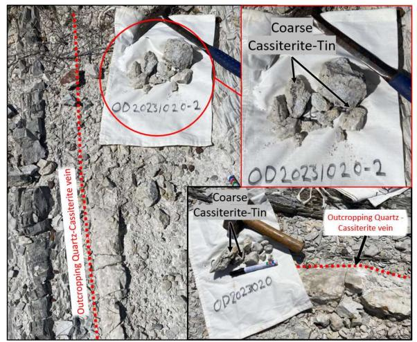
Figure 2: Tallebung Tin Project – Rock chip samples pictured next to the outcropping quartz veins sampled.
