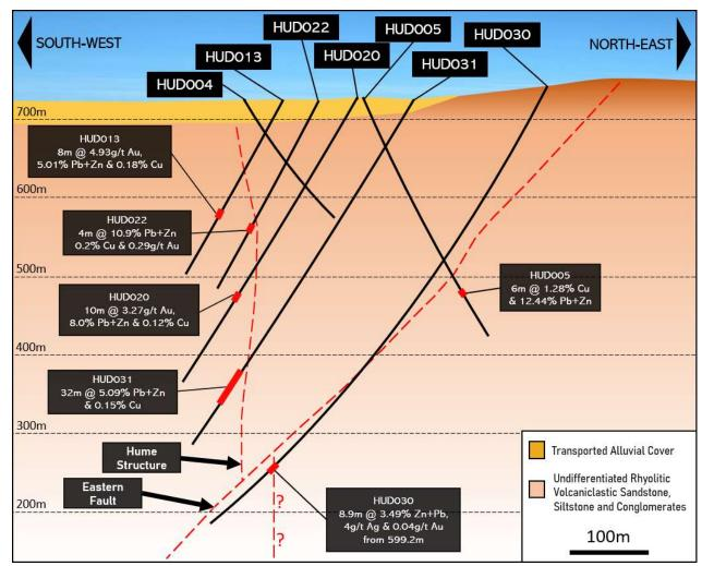
Figure 6: Hume Target – Cross-section of HUD030 showing the trace in red of the extension of the hole to test the Hume Structure at depth and provide a platform for DHEM – Assays are pending for the extended hole interval shown in red.
