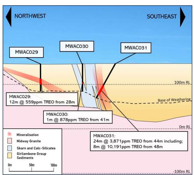
Figure 3: Doradilla Project – Cross-section from MWAC029 to MWAC031 showing the DMK line Skarn above the Midway Granite with the Midway Granite coming to surface and outcropping to the northwest.
