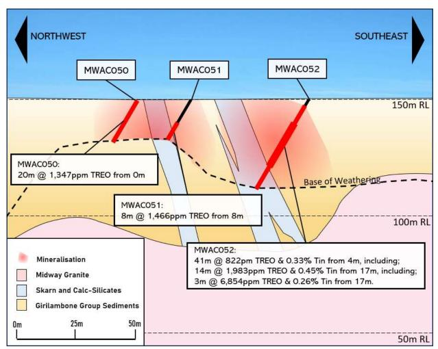
**Figure 4:** Doradilla Project – Cross-section from MWAC050 to MWAC052 showing the multiple skarns of the DMK line associated with REE and tin mineralisation above the Midway Granite which underlies the area.
