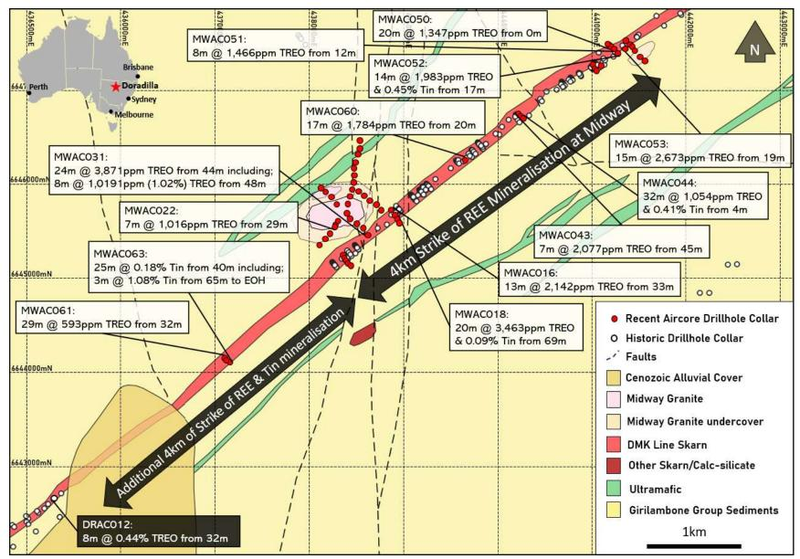
Figure 2: Doradilla Project – Map shows the large strike extension of the previously undrilled and untested strike between Midway and Doradilla on the DMK Line and the previous strike extent with recent aircore drilling intercepts overlaid on the mapped and interpreted geology.
