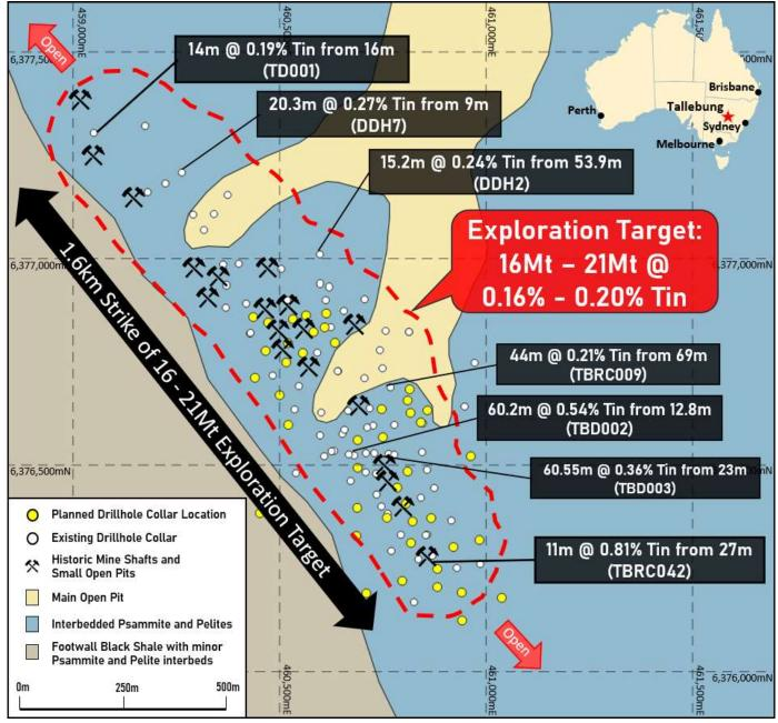
Figure 1: Tallebung Tin Project – Plan view showing the past drilling with highlighted intercepts, the extent of the current Exploration Target and maiden MRE, along with the locations of the planned drillholes in the resource expansion and infill drilling program now commenced overlaid on the geology.
