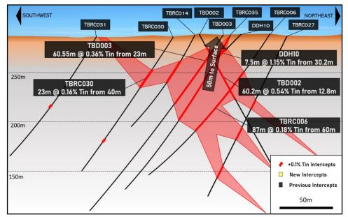
Schematic Cross-Section of Shallow High-Grade Zone
