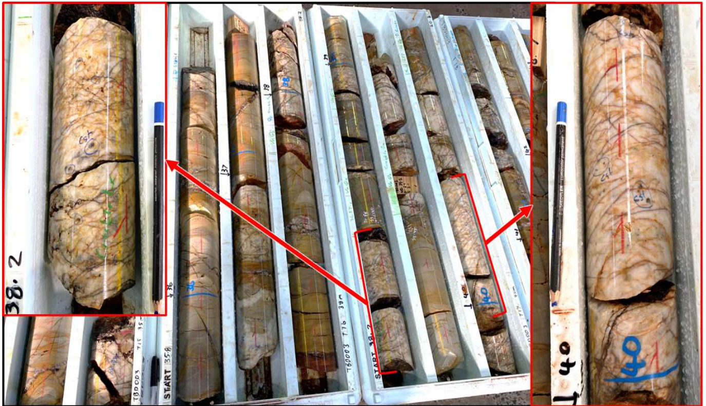
Figure 4: Tallebung Target – Drill core from the first diamond hole in the latest program, TBD003 (33.3–43.05m), intense quartz veining hosting abundant cassiterite (tin oxide). Left-hand side red box: a close up of 38.2–38.4m – visible coarse cassiterite circled in blue chinagraph, hosted in a large quartz vein. Right-hand side red box: a close up of 40.0–40.3m – coarse cassiterite up to 10mm across circled in blue, hosted in a quartz vein. Core is 83.1mm wide for scale. NB: Cassiterite contains over 78% tin and is 2.6x denser than quartz, therefore, 1% cassiterite in the core = over 2% tin grade.
