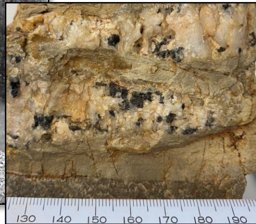
Cassiterite Ore from Tallebung Scale in mm
