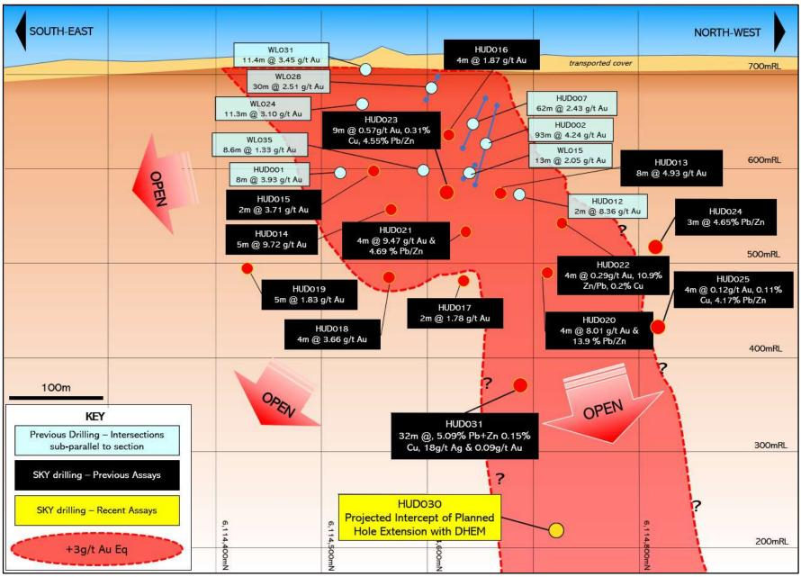
**Figure 9**: Hume Target – Schematic long-section with significant intercepts.
