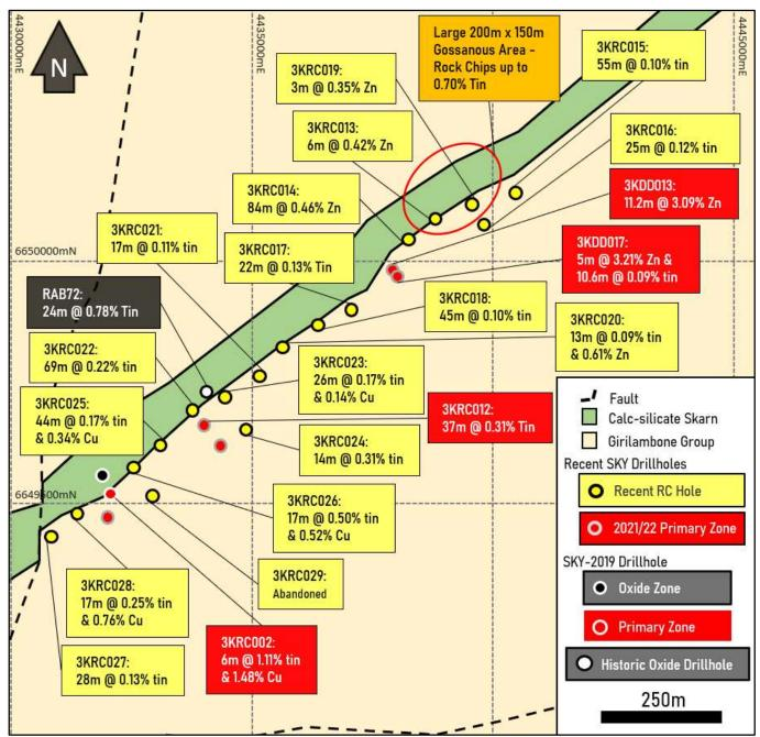
*Figure 6: 3KEL Target – Plan view showing the past drilling with the recent RC drillholes. Recent results are in yellow, past results in red and black for oxide and primary intercepts, respectively.*
