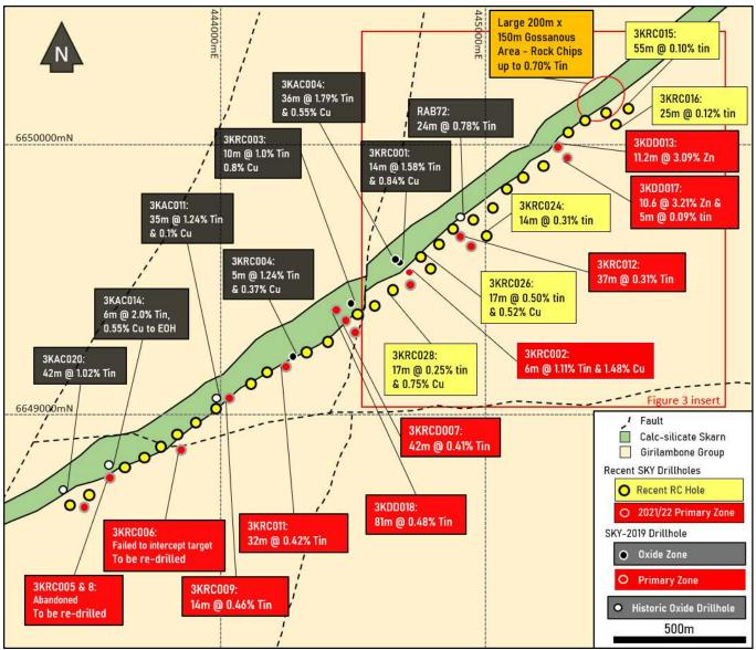
*Figure 5: 3KEL Target – Plan view showing the past drilling with the recent RC drillholes. Recent results are in yellow, past results in red and black for oxide and primary intercepts, respectively.*
