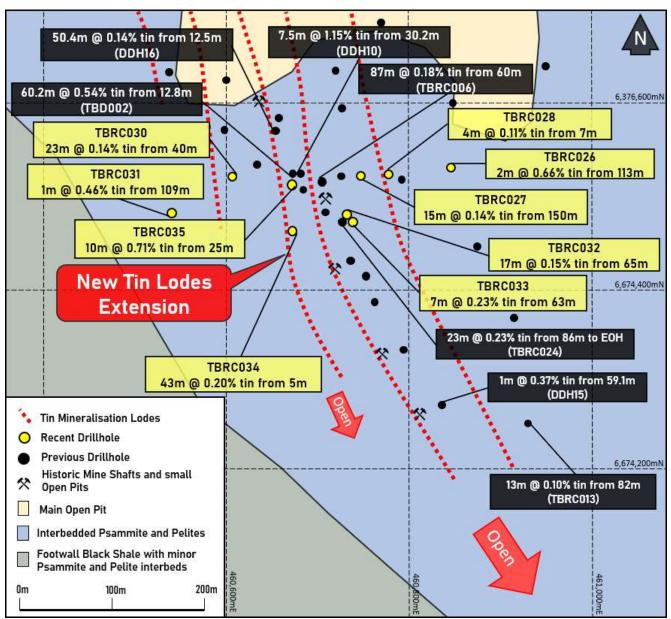
Figure 3: Tallebung Target – Plan view of the southern area of the Tallebung Target showing the new lode extended by new hole TBRC034, adding significant new tin mineralisation to the Tallebung Target. Recent holes are in yellow
