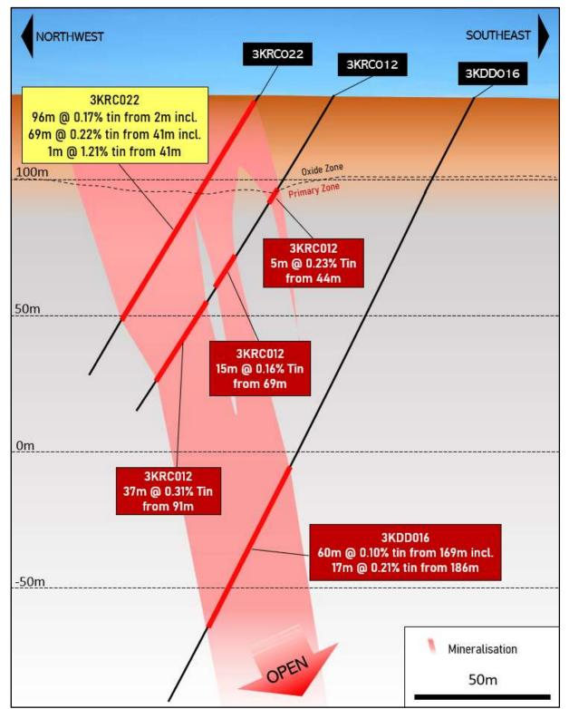
Figure 7: 3KEL Target - Cross section of 3KRC012, 3KDD016 and recent hole 3KRC022, recent results are in yellow.
