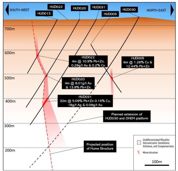
*Figure 8*: Hume Target – Cross-section of *HUD030* showing the trace in a dotted line of the planned extension of the hole to test the Hume Structure at depth and provide a platform for DHEM.
