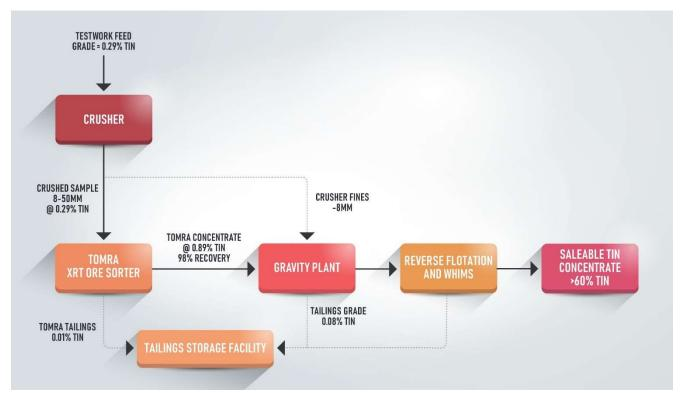
*Figure 4:* Tallebung Target – Simplified schematic flowsheet starting with the TOMRA XRT Ore Sorter to increase the tin grade and significantly reduce the total mass to undergo further processing. The TOMRA concentrate then gets further upgraded in the gravity plant before reverse flotation and WHIMS dressing to produce the saleable tin concentrate.
