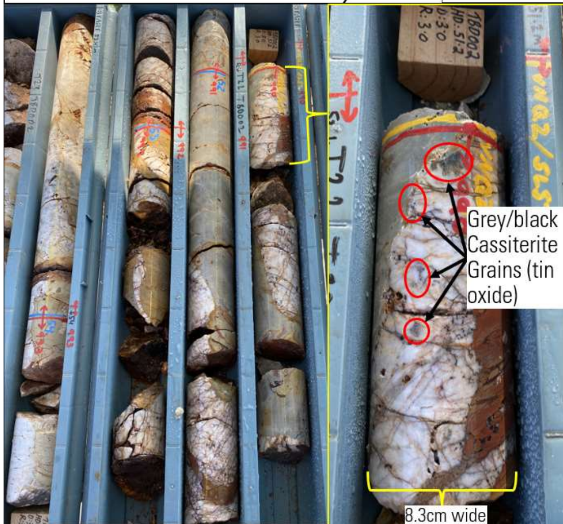
Figure 7: Talbung Target – Top -Cross-section showing the position of TBD002 ; Bottom Left - TBD002 drillcore 51.2-54.2m with intense quartz-cassiterite veining; Bottom Right - Close up of TBD002 51.2-51.4m with large visible cassiterite (tin oxide) grains circled in red.
