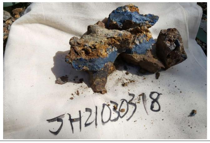
**Figure 2** – **EL6064 - Monarch** – 26.1% Cu, 0.41 g/t Au, 29 g/t Ag. Spectacular assay result from the >1cm azurite vein and may also contain some chalcocite. Width of view 20cm.
